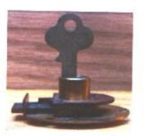
tube & plug. When the blank fits in the lock, mark the outside of the blank, and file the throat cut from this mark (towards the tip) until the blank turns in the plug. Remove the
